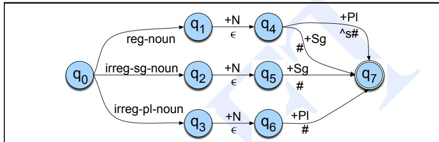
**Figure 3.13** A schematic transducer for English nominal number inflection  $T_{num}$ . The symbols above each arc represent elements of the morphological parse in the lexical tape; the symbols below each arc represent the surface tape (or the intermediate tape, to be described later), using the morpheme-boundary symbol  $\hat{\ }$  and word-boundary marker #. The labels on the arcs leaving  $q_0$  are schematic, and need to be expanded by individual words in the lexicon.
