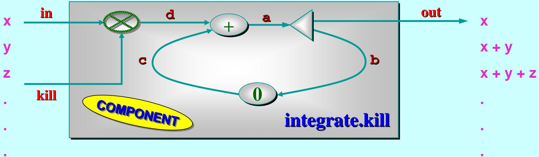
To shut down a network *gracefully* (without leaving some processes stranded – i.e. deadlocked), we *poison* all the components. The poison spreads through the normal dataflow.
