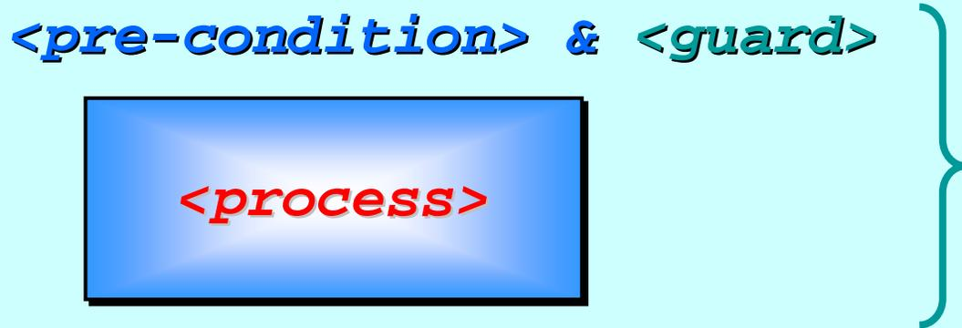
For each execution of an **ALT** (or **PRI ALT**), any *pre-conditions* only need evaluating *once* – no rechecks are necessary.
