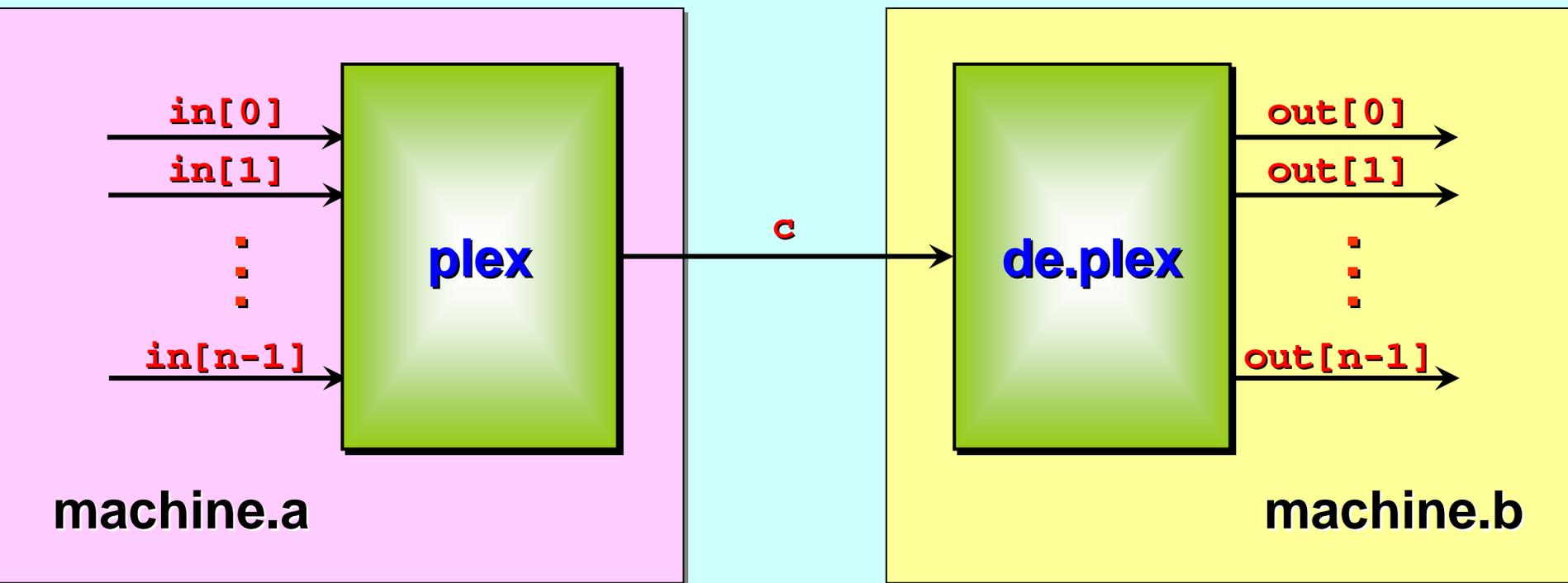
If each *message* arriving at **plex** (and departing **de.plex**) is of type **THING**, then each *message* on the *multiplexed* channel consists of a channel array index (type **INT**) followed by a **THING**.
