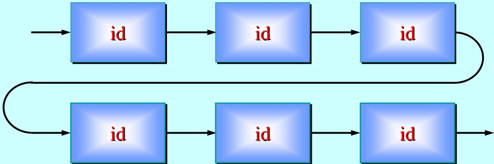
is a blocking *FIFO* buffer of capacity 6
