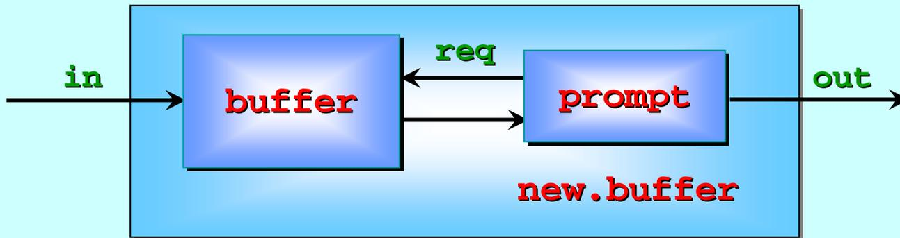
Just as when used like this with the **mem.cell** process, **prompt** holds old (*stale*) data. Meanwhile, the **buffer** holds anything new that arrives. *This is a good thing this time!*
