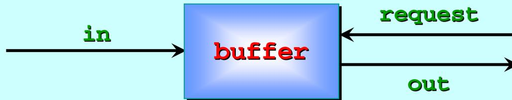
**buffer** has a capacity of **max** (say). A process may send data into the buffer until it is *full*. If it then tries to send more, it will be blocked until the buffer gets emptier.
