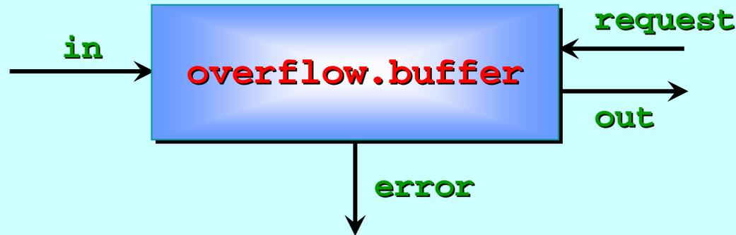
This is the same as **buffer**, except that it does not block the source when it is full. Instead, it outputs a signal on the (**BOOL**) **error** line and discards the incoming item.
