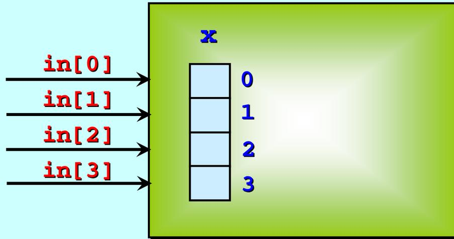
Before, we introduced the *replicated* **PAR** for this. We knew that a message on *one* channel was accompanied by a message on *all* channels.
