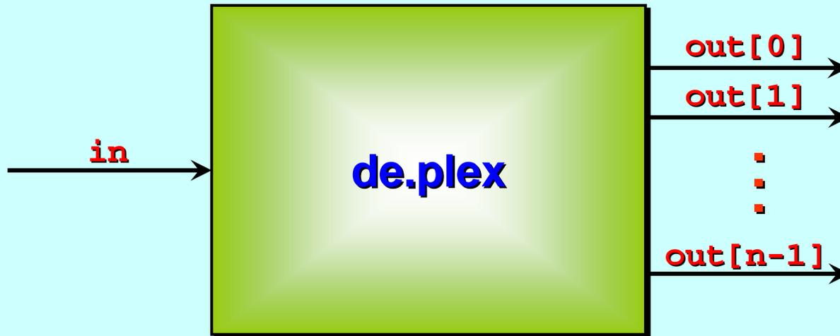
This process recovers input messages to their correct output channels ... and assumes each message is prefixed by the correct target channel index ...
