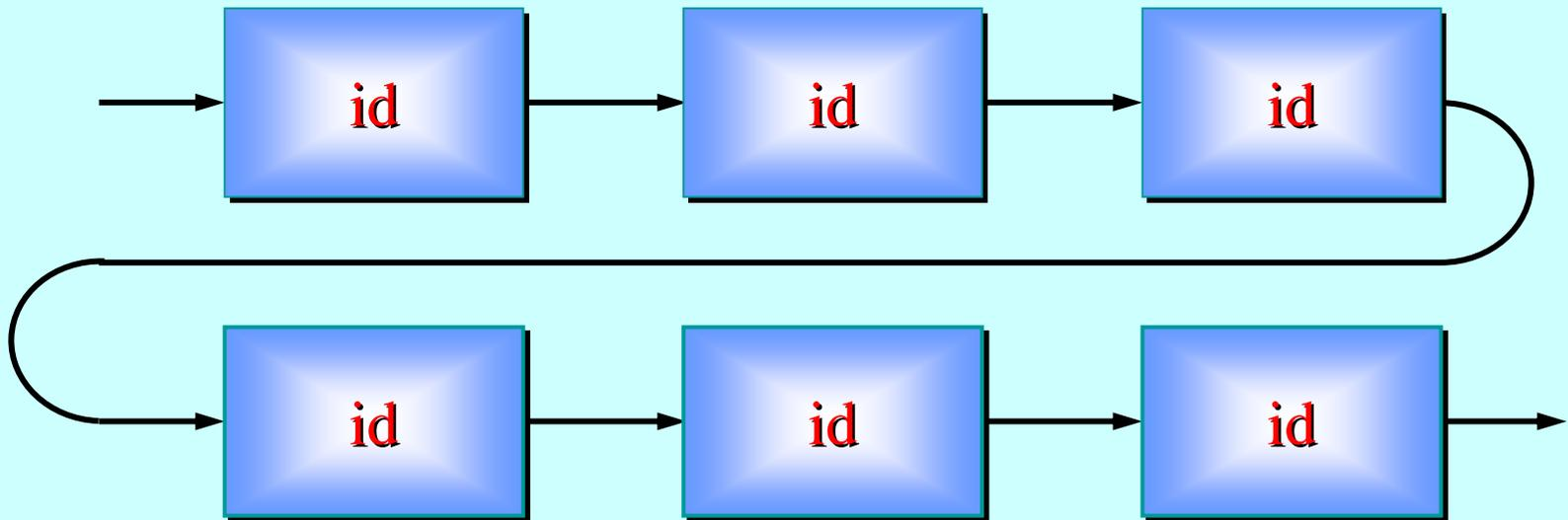
... but not so good *for software* ... where each item of buffered data must be copied (from process to process) **N** times (where **N** is the size of the buffer).
