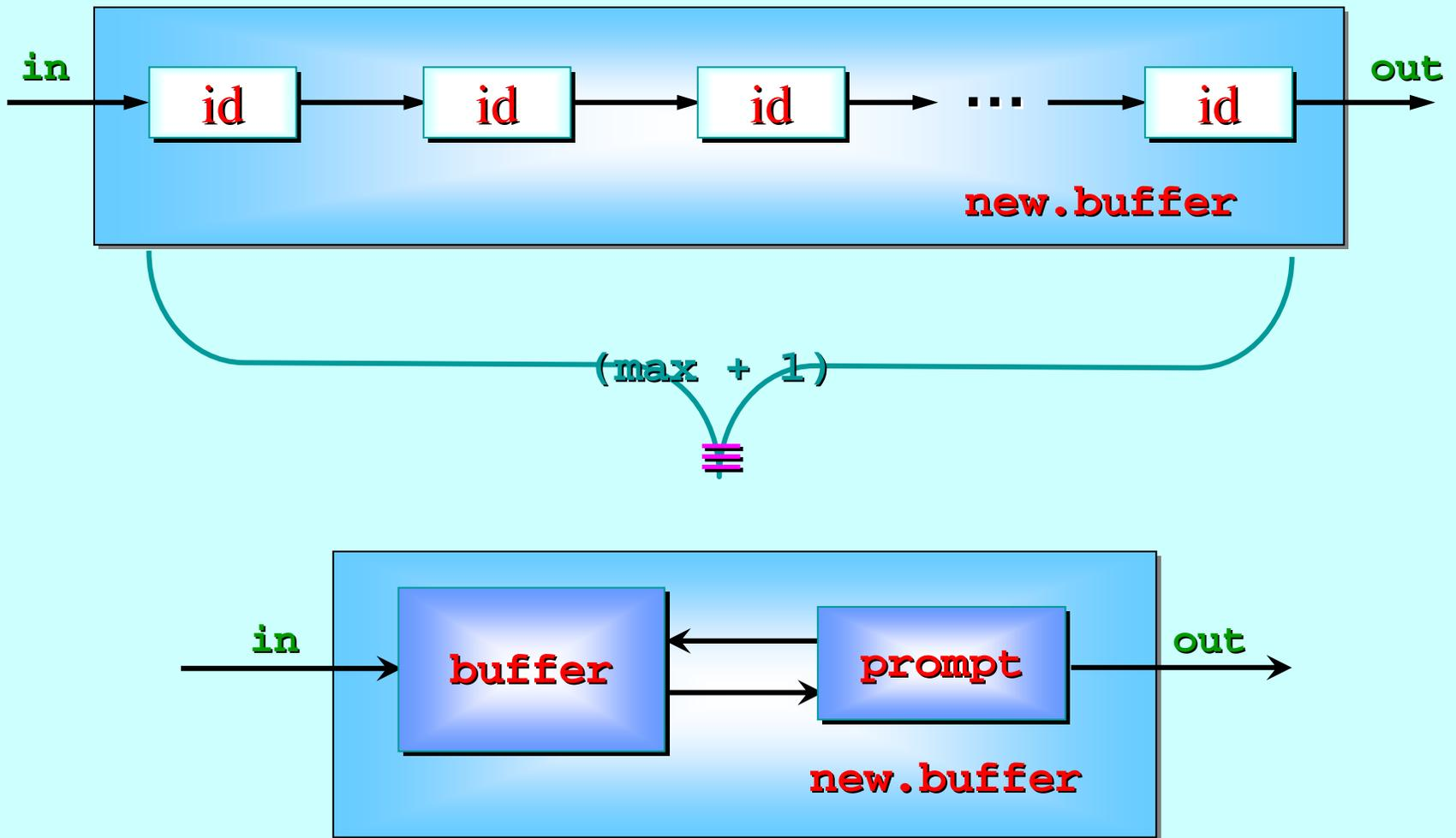
The top version is a more regular and simpler design. The bottom is more efficient for software – less copying of data.
