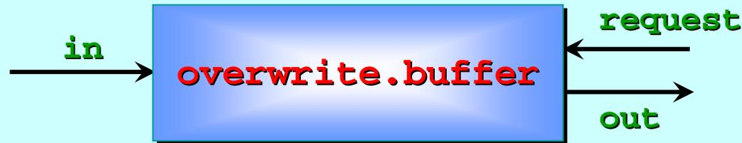
This is similar to `overflow.buffer`; it also does not block the source when it is full. However, the incoming item (when full) is not discarded but *overwrites* the oldest item in the buffer. No error is reported for this (though another version could easily do that).
