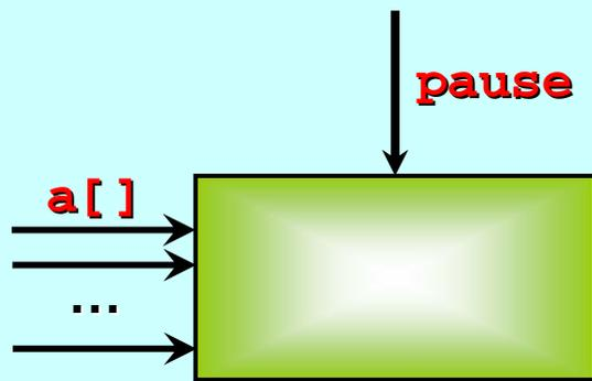
**ALTing** between *an array* of channel inputs, *a single* channel input and *a single* timeout.
