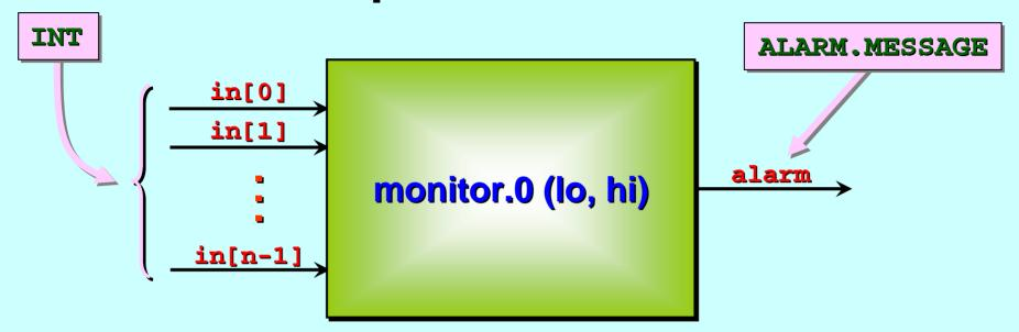
The input channels deliver raw sensor data (such as *temperature/pressure* measurements from a machine). The rate of supply of this data is *irregular*.
