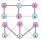
Mark the source, A, with color1, mark the nodes at level 1 with color2, and so on. Every node on an even numbered level will be color1 and every odd color2
