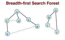
Tree edges are solid lines and dashed lines are cross edges.
