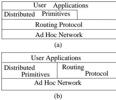
Figure 1. Two possible approaches for implementing distributed primitives.
